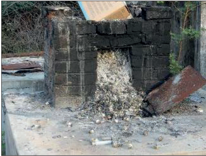
Low Temperature Brick incinerator used for burning syringes
