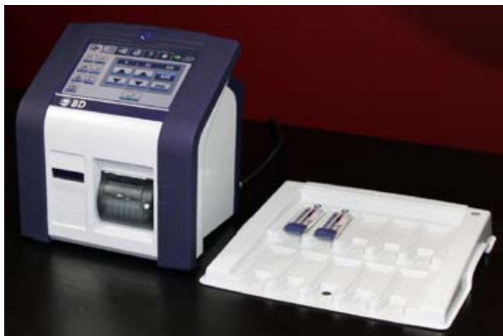
POC CD4 Device from BD Biosciences. Photo source: BD Biosciences.
