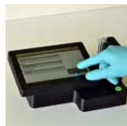
Bottom, left to right: 1) Inserting a single-use EOSCAPE cartridge into processing unit; 2) fingerstick sampling directly into the cartridge; 3) scanning test results with EOSCAPE touchscreen analyzer.
